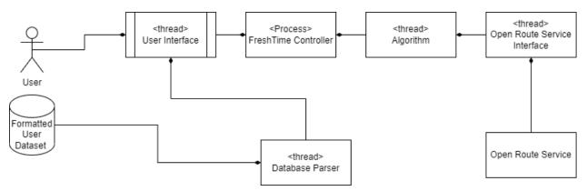
This shows how the system is made up of individual processes that spawn threads which perform a specific task.
